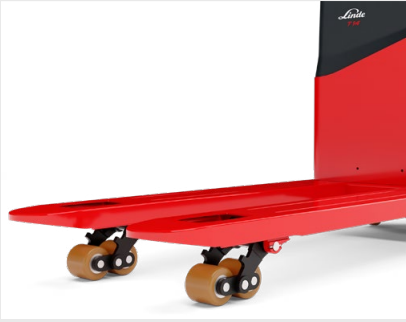
Castor wheels for additional stability
