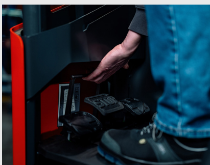
Height-adjustable pedal plate for maximum comfort
