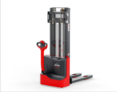
Long tiller arm and emergency stop switch
